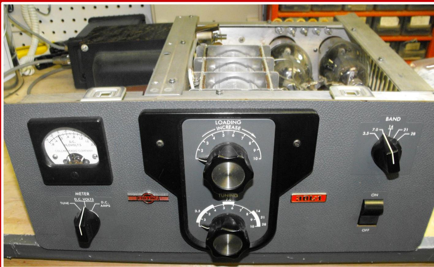
COLLINS PROMOTIONAL TEXT - "The Collins 30L-1 has 1000 watts PEP power input on SSB and 1000 watts average on CW on 80, 40, 20, 15 and 10 meters. Uses TWO FINALS (811A) Drive power is 70 to 100 watts for full power output. RF connection is N type."
