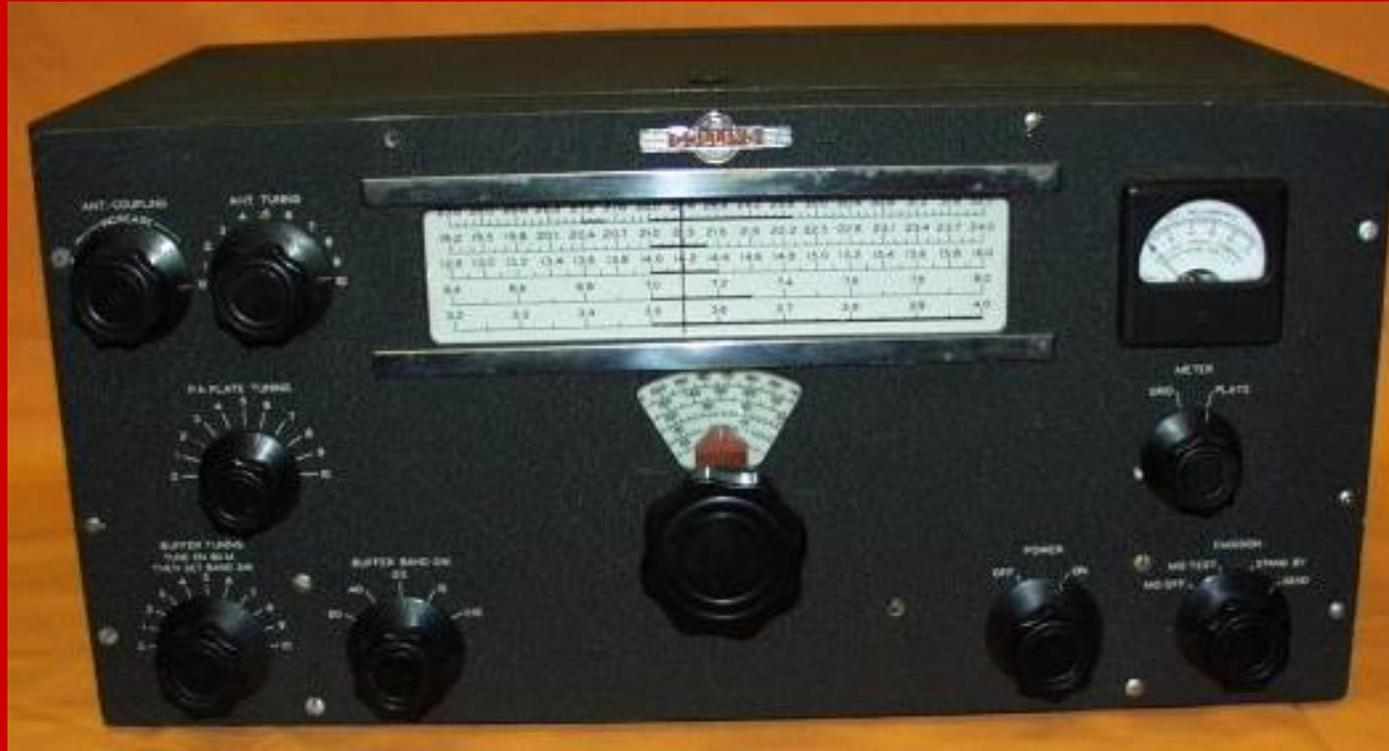
***Collins promotional text about the 310's*** - "The Collins PTO (permeability tuned oscillator) exciters give you not only the flexibility and convenience of variable frequency, but also the accurate calibration and high stability inherent in the Collins 70E-8A-PTO.." - Ran 40 watts
