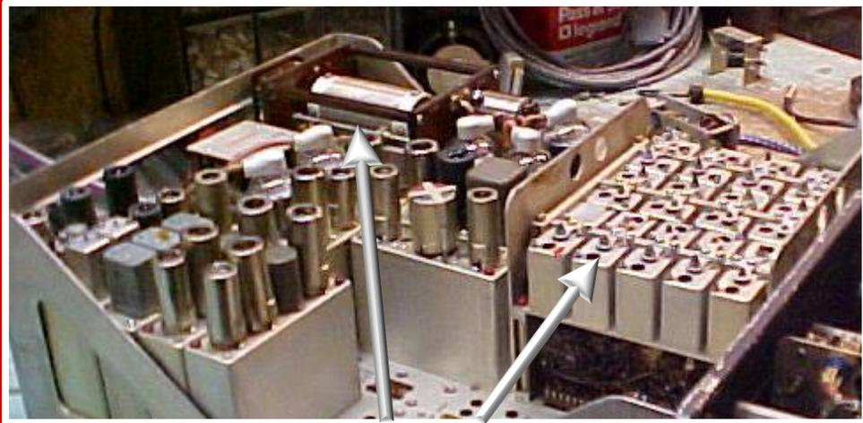
Can Slugs and PA Coil AutoTuned for Each Crystal
