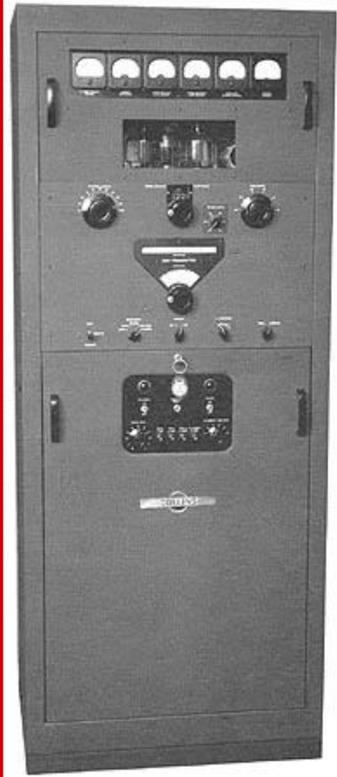
COLLINS PROMOTIONAL TEXT - "The KW-1 is a vfo controlled, band-switching, gang tuned, phone and cw transmitter. Its input is a full 1000 watts on the 80, 40, 20, 15, 11, and 10 meter bands and 500 watts on the 160 meter band. The entire transmitter together with its power supply is enclosed in a handsome grey, wrinkle-finish cabinet."
