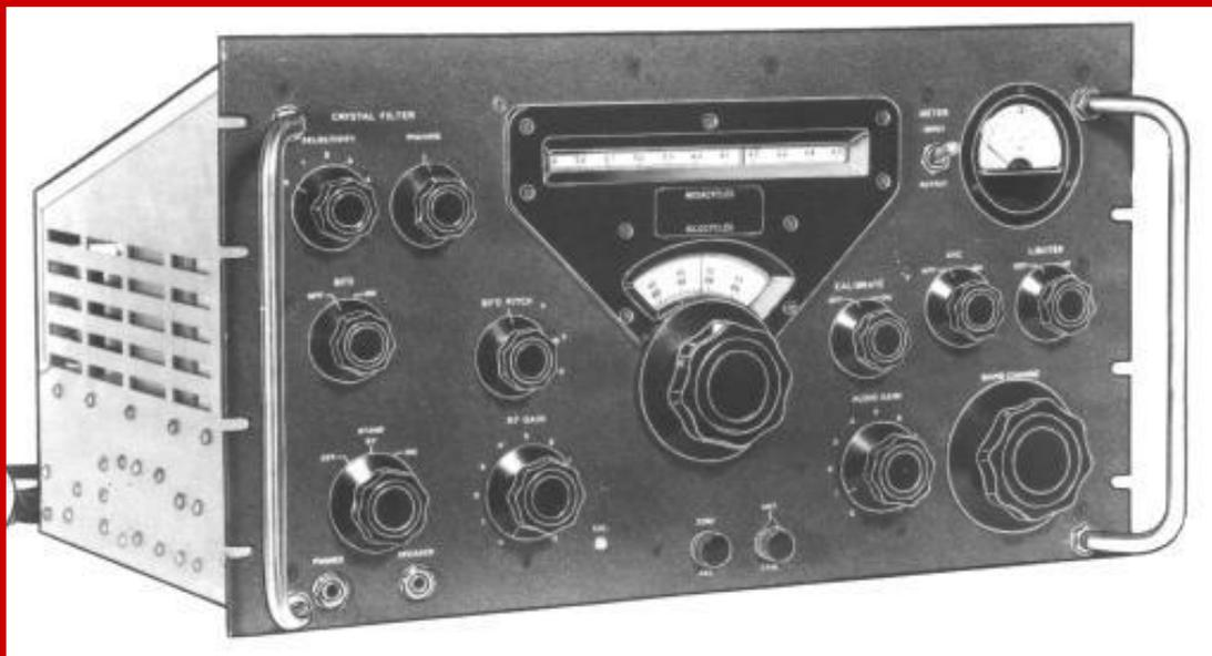
“The Collins 51J-4 Receiver is designed for communication applications where stability and dial accuracy of the highest order are the prime requisites. Under normal operating conditions, the receiver operates in the range of 540 kc to 30.5 mc with a total setting error and ***drift of less than 1 kc at any frequency within its range***. This receiver incorporates the new mechanical filter in the intermediate frequency range to obtain the desirable rectangular- shaped passband.
