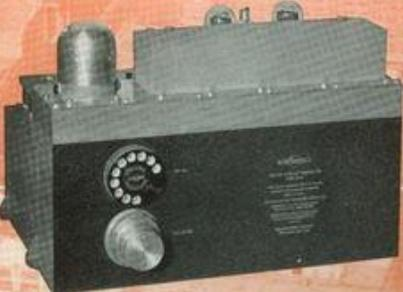
AUTOTUNE – “Proved to be one of the most significant developments in the success of Collins Radio Company.” In the initial stages of equipping aircraft with radios was changing the many channels needed for communication. Each new frequency required retuning. Braniff for instance didn’t want to pay for extra radio ops to tune the radios. Collins responded to this need with the mechanical AutoTune function. It helped bring an Allied victory in WWII.
