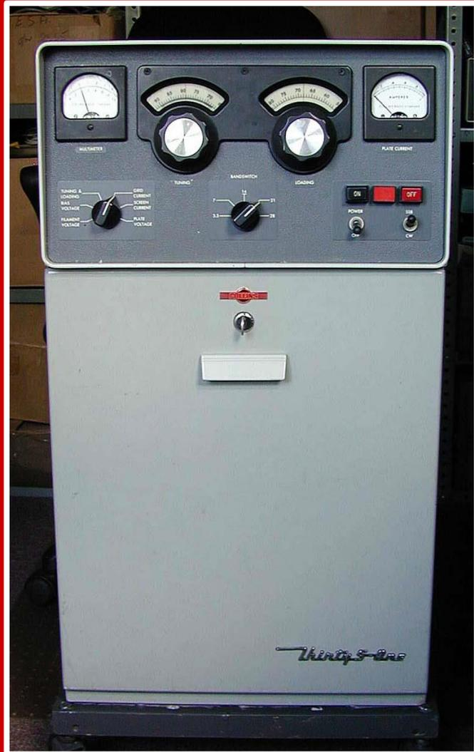
The Collins 30S-1 is a single final tube (Eimac 4CX1000A), grounded grid linear amplifier with frequency coverage consistent with the 32S-1 and 75S-1. It provides full legal power input for SSB (1kW average) or 1kw input for CW, requiring 70 to 100 watts excitation. By retuning the input coils as necessary other frequencies are available in the range of 3.5-5 and 6.5-30 MHz.
