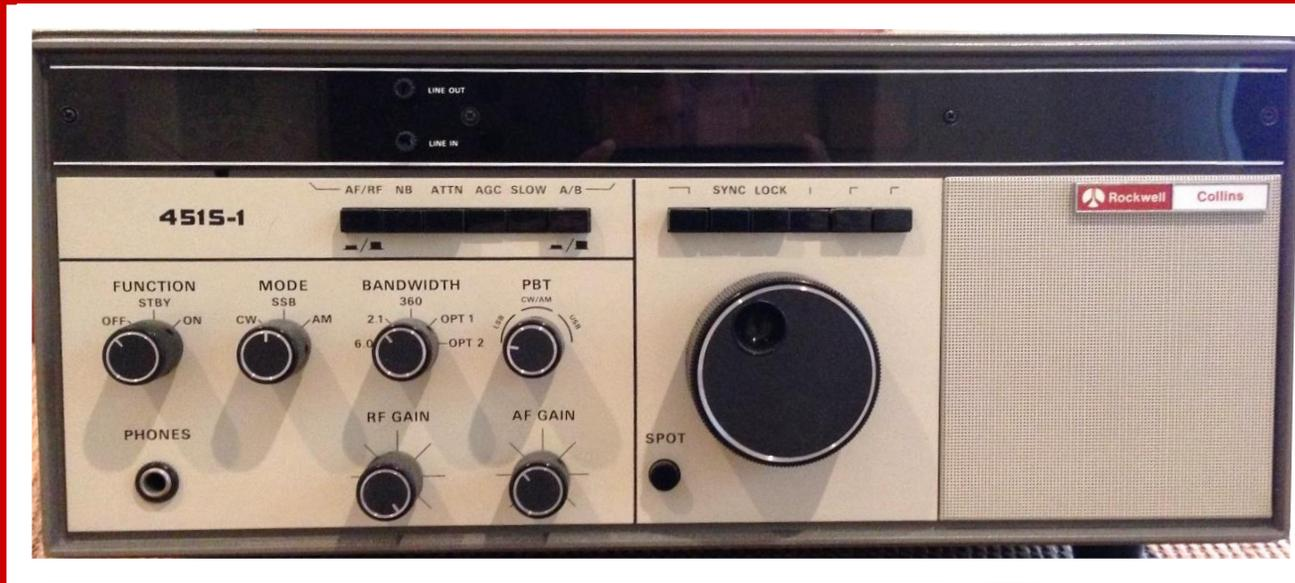
“The 451-S is a professional single sideband (SSB) communications receiver that offers reception of upper and lower sideband, CW, AM, or FSK signals over the frequency range of 0.2 to 30 MHz. The unit is of *solid-state design* ... and uses single knob tuning to cover the entire frequency range without band switching. A high resolution *synthesizer with microprocessor* controls four tuning rates down to 10 Hz increments.”
